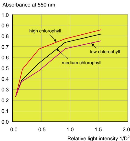
**Figure 6** Graph to show the absorbance (at 550 nm) in relation to light intensity of balls made of three different concentrations of algal cells.
