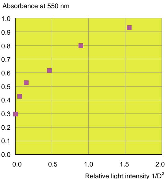
**Figure 4** Graph to show the absorbance (at 550 nm) of indicator from six vials over a range of light intensities. Light intensity was a relative measurement calculated as  $1/(\text{distance})^2$ .
