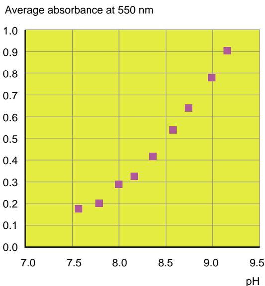
**Figure 2** Graph to show the absorbance at 550 nm of pH buffers ranging from 7.6 to 9.2 with added hydrogencarbonate indicator.
