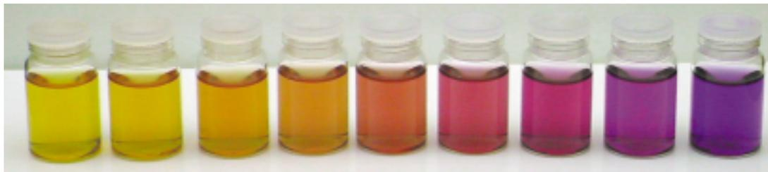
**Figure 7** Buffer solutions ranging from pH 7.6 to 9.2 (at intervals of 0.2). 9 cm<sup>3</sup> of each buffer solution was mixed with 1 cm<sup>3</sup> of stock hydrogen carbonate indicator.
