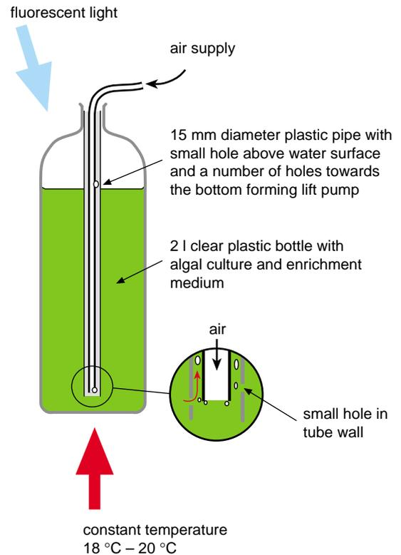
Figure 1b A simple algal generator showing the operation of a lift pump.
