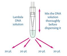
Use a new tip to add the DNA solution to each tube, to prevent contamination
