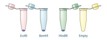
As you add the DNA solution to each tube, mix it gently so that the dried restriction enzyme dissolves completely
